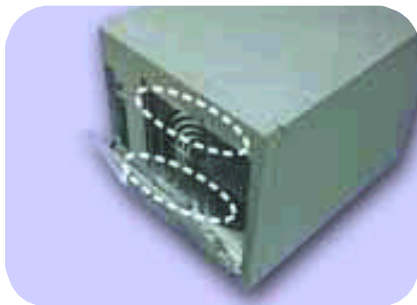
Well Shielding for EMI solution
