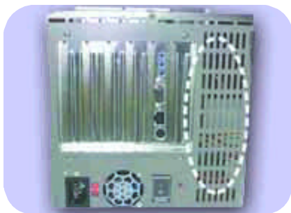
Better ventilation and high frequency CPU thermal issue
