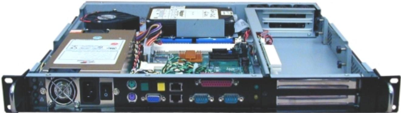
The innovative ITOX Expanding Dragon 1U rackmount server meets industrial computer requirements for processing power, multiple expansion slots, storage, advanced cooling, and low cost. ITOX offers the Expanding Dragon as a barebones platform (case, power supply and motherboard) or a full system (including CPU, memory, hard drive and operating system). Both quality-built designs support high density, industry-standard rackmount applications.
