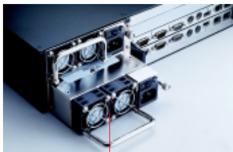
300 W 1+1 redundant ATX power supply
