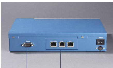
RS-232 console port Three LAN ports
