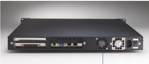
Rear-end 10 CFM cooling fan
